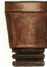
Tapered sabot for howitzers – necessary as the powder chamber was smaller than the bore
